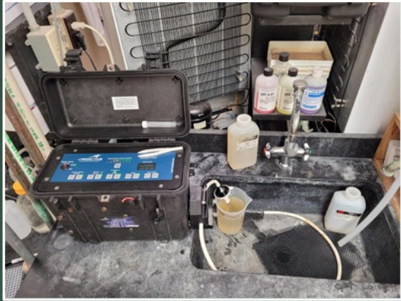
Filtration Peristaltic Pump & Smith- Root eDNA glass filter pack
