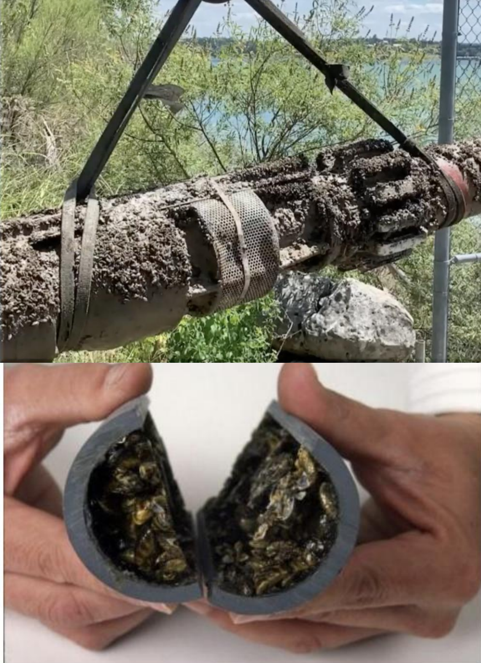
Figure 2: Zebra Mussels in Small-Diameter Pipe (Source: Associated Press, 2014)
