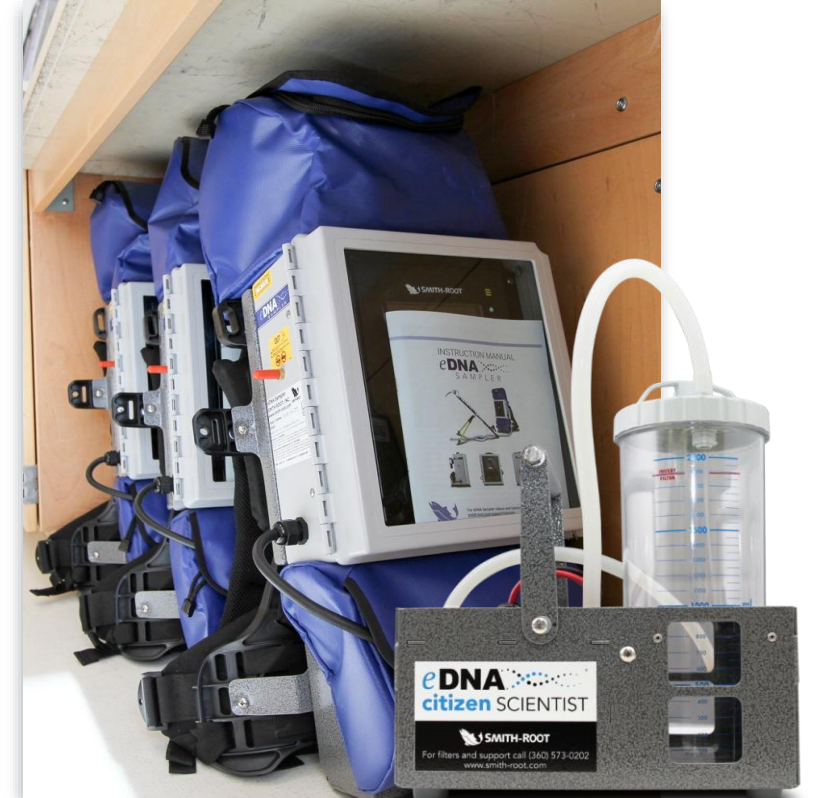
eDNA Sampling Equipment Smith-Root eDNA backpack samplers
